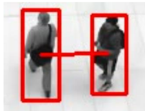
Figure 3. The Result of Object Detection and Define a Centroid Point between Two Objects
