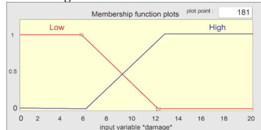
Figure 6. Degree of Membership of the Damage Variable
